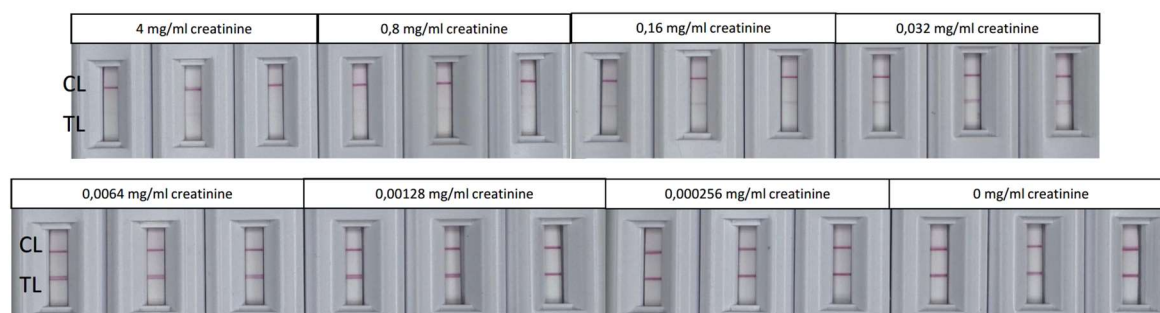
Figure 58: Lateral flow assay for the detection of creatinine
