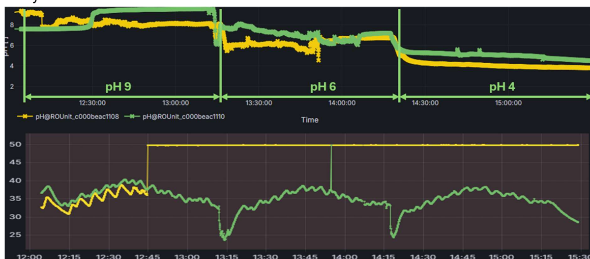
Figure 100: pH and temperature curves of TNO / CSEM sensor flex. The sensors are able to detect the pH and temperature levels quite well. Jagged lines on the temperature measurements might be due to the controller of the heating elements overshooting slightly.
