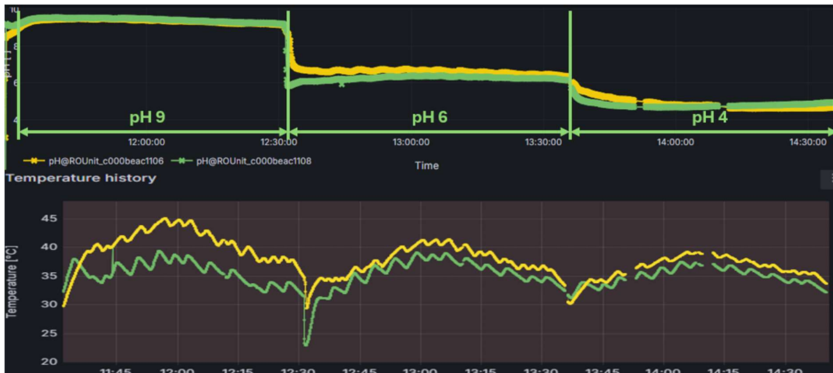
Figure 101: pH and temperature curves of addensors / Würthsensor flex.
