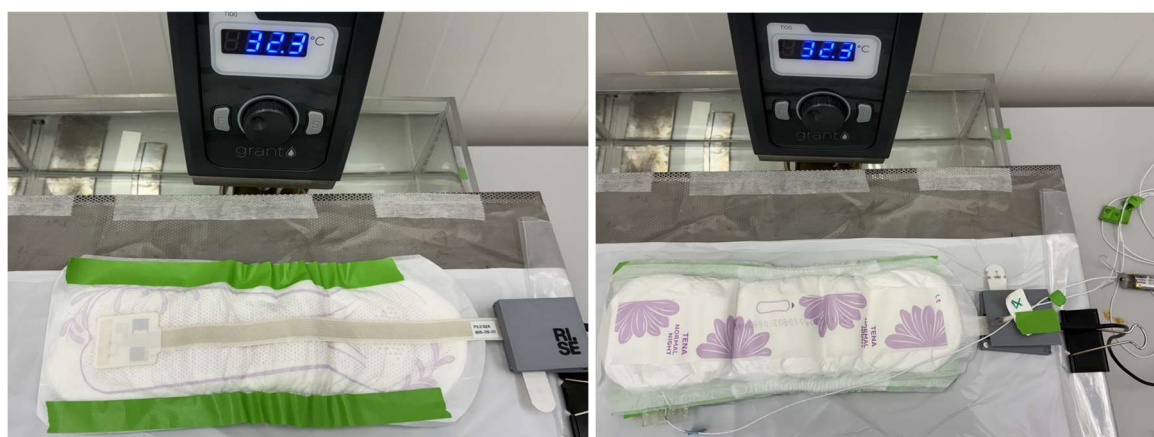
Figure 78. Testing of sensor labels with water-bath at ESS. (left) A sensor label mounted on the incontinence material. (right) Reference temperature and humidity sensors attached near the sensors on the sensor label and outside the incontinence material.
