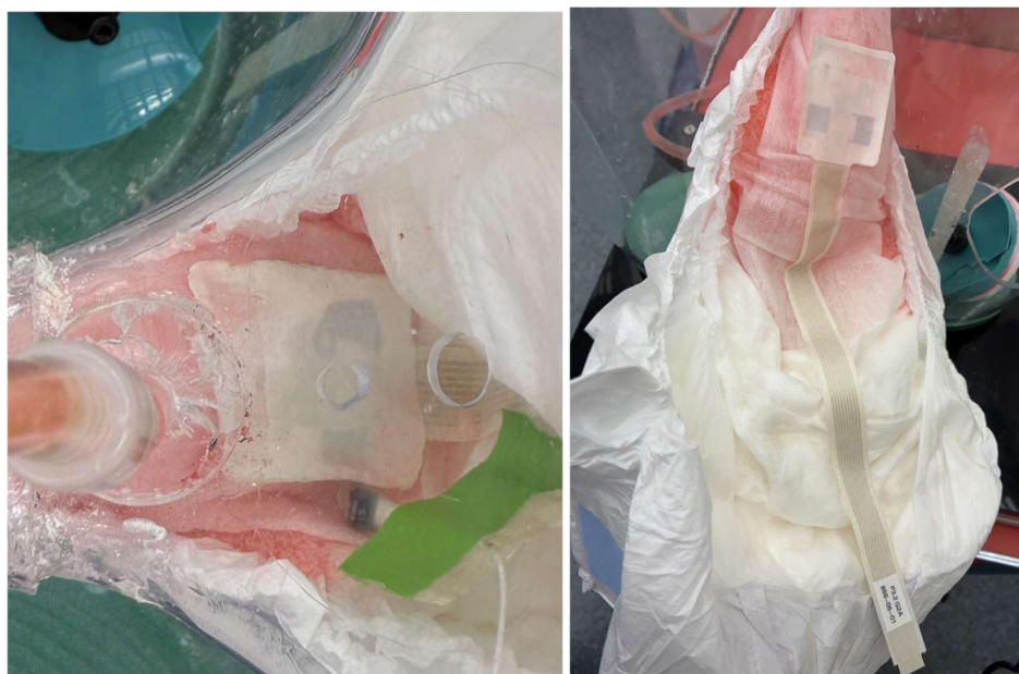
Figure 80. Left: A close-up of the dispersion of the urine inside the incontinence product where the sensor label and reference sensors are placed. Right: A view after the test.
