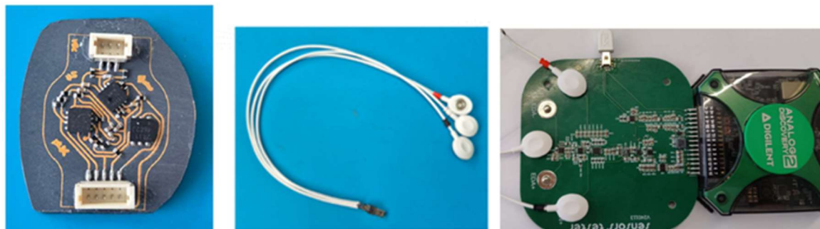
Figure 18: Sample 3 of EEG LDS PCB prototype / PLUX EEG sensors to connect with the PCB / test setup
