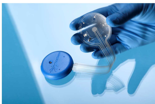
Figure 86 In blue reusable readout unit and on flexible PET the research platform for sensor integration comprising more than seven positions for sensors.
