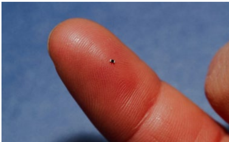
Figure 31. Perspective of the 0402 component to be assembled in the circuit produced by LDS.
