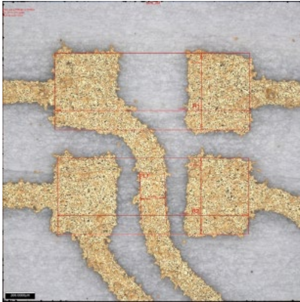
Figure 32. Microscope image (2 x 2 mm) showing the circuit track with thickness of 0,16 mm passing through a 0402 component (1 x 0,5 mm).
