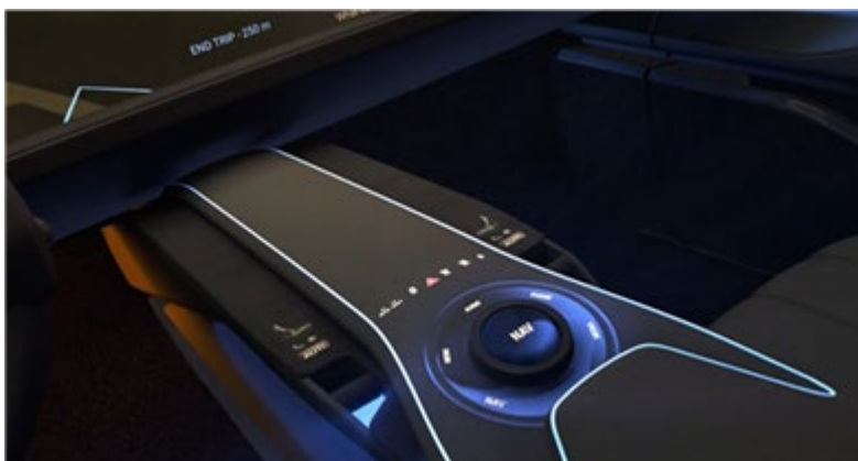
Figure 7: Example of an IME Automotive control panel.
