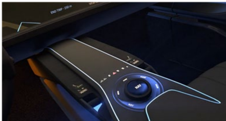
Figure 7: Example of an IME Automotive control panel.
